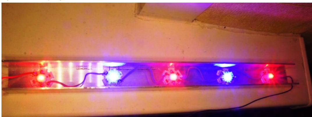
Fig. 1. Sectional panel with light emitting diodes of blue and red colors
